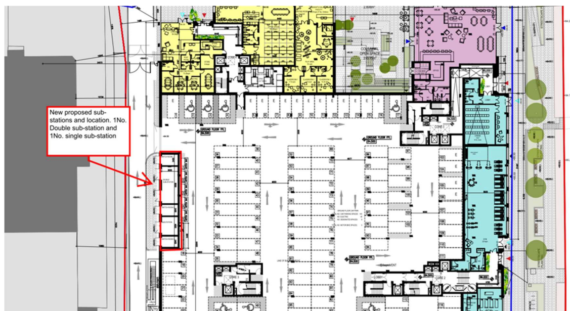
Fig 1.1 ESB substation in new development
